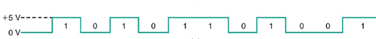
Digital signals (a) Telegraph (Morse code). (b) Continuous-wave (CW) code. (c) Serial binary code
